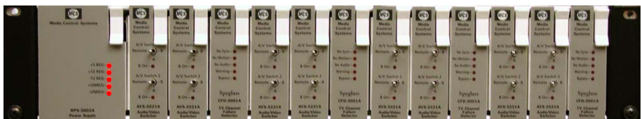
6-Channel 2-RU Chassis, Four Channels Shown with Video and Balanced Stereo + SAP 2x1 Switching
